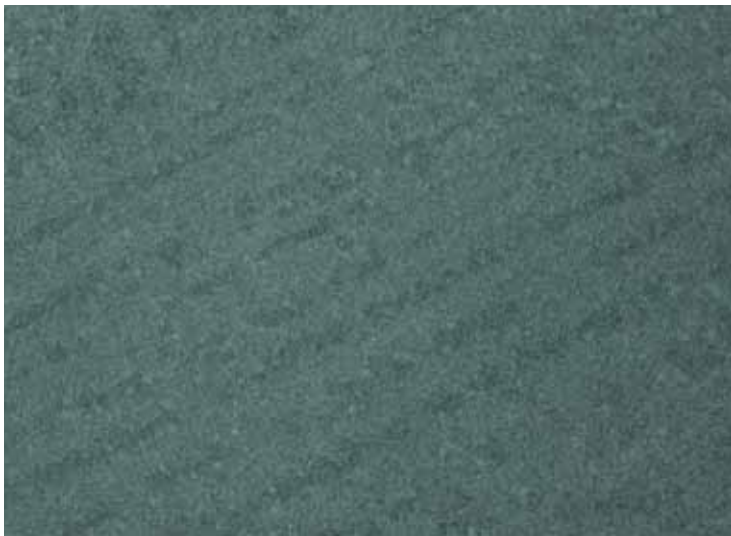
SANDED: The top surfaces of sawn slabs are coarsely diamond sanded to produce a non slip finish.
