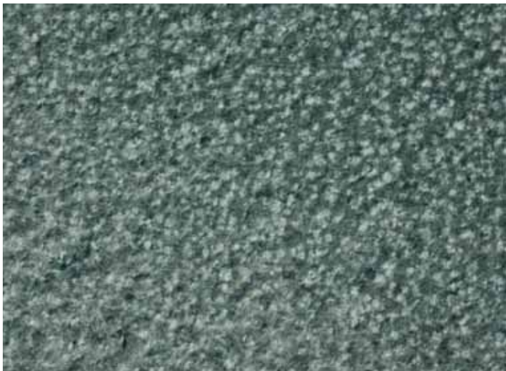
SPOT TEXTURED: The top surfaces of sawn slabs are pneumatically tooled to produce a pitted surface.
